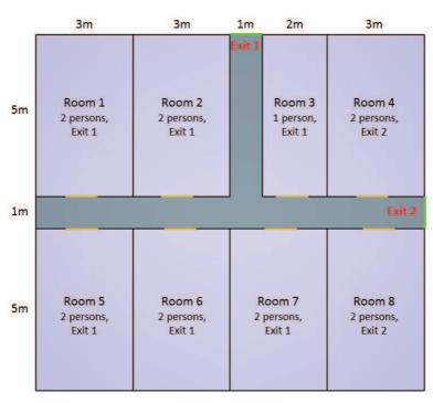
Fig. 1. Room arrangement in the test case
