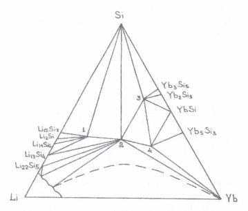
Fig. 1 Isothermal section of the Li-Yb-Si system at 470K (1 -  $\sim$ Li<sub>10</sub>Yb<sub>3</sub>Si, 2 - LiYbSi, 3 - Li<sub>0.3</sub>YbSi<sub>1.7</sub>, 4 -  $\sim$ Li<sub>2</sub>Yb<sub>5</sub>Si<sub>3</sub>)
