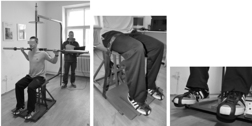
Figure 1. Assessment of trunk rotational power and velocity using the FiTRO Torso Isoinertial Dynamometer.
